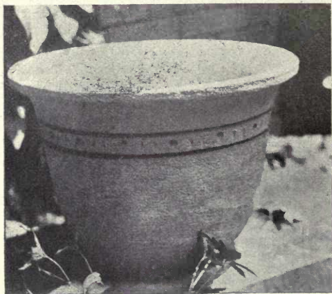
FIG. 62—GOOD DESIGN AND INTERESTING TEXTURE; DRY-TAMP CONCRETE IN PLASTER MOLD—PHILADELPHIA SCHOOL OF INDUSTRIAL ART
